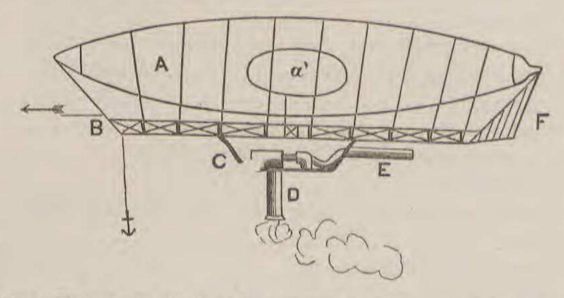
A, balloon ; B, upper deck ; C, lower deck for machinery ; D, smoke stack ; E, nozzle ; F, rudder ; a', interior air-sack.
